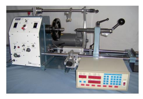
The new GORMAN HDH CNC HAND WINDER is an all-in-one winding machine which will wind about any coil imaginable, depending on the ingenuity of the operator. Wires from the finest, to as heavy as number 4 AWG, are handled with equal ease with the two speed ranges and CNC Controller.
