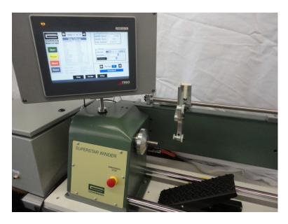
Gorman Machine Corp has developed the new SuperStar Winding Machine for the purpose of having a machine that can handle all the unique winding requests we previously could not offer. The new Trio Controller in combination with the 10" Trio HMI controls the following winding functions.
