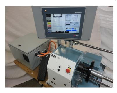
Gorman Machine Corp has developed the new Super HDH Winding Machine for the purpose of having a machine that can handle all the unique winding requests we previously could not offer. The new Trio Controller in combination with the 10" Trio HMI controls the following winding functions.
