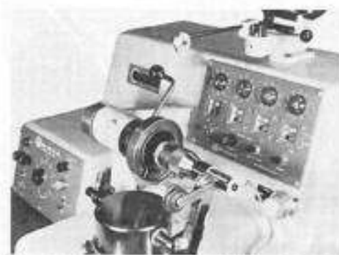
Fig 4 Combination toroidal and bobbin winder shows the equipment set to wind bobbins. Operator can change the head quickly with assemblies of various sizes to produce toroids.
