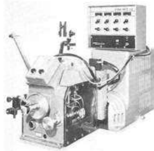
Fig 3 Typical single spindle machine set up to wind bobbins.
