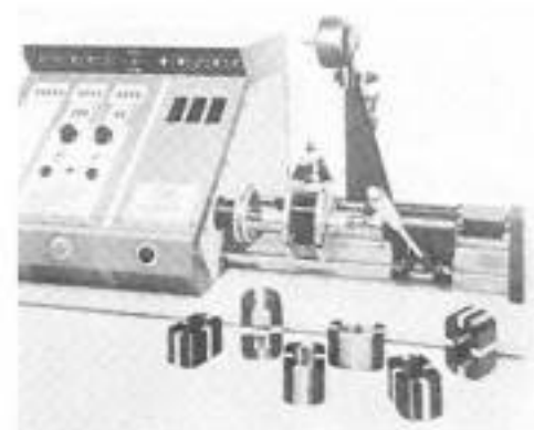
Fig 2 Lathe-type winder manufactured by Eubanks Engineering makes perfect layer coils. Note hysteresis tensioner for wire feed.
