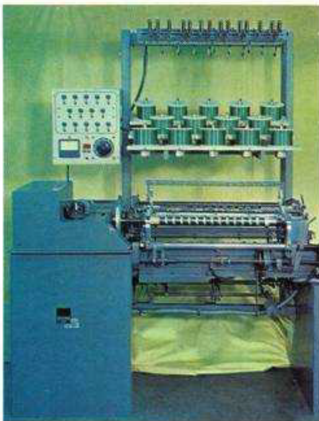
Coil winder operates up to 2500 rpm, accepts up to 15 inserts per minute. Leeson Corp.
