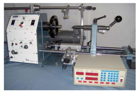
Our standard HDH CNC Heavy Duty Winder has Two Speed Ranges. A Low Speed Range for wire as heavy as 4 AWG and a High Speed Range for wire to the finest sizes. With the flip of a toggle switch you can seamlessly change speed ranges without stopping the machine through the use of internal clutches. No Back Gears to engage. The toggle switch middle neutral position allows for hand turning the spindle.
